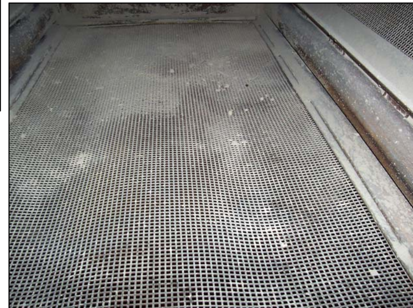
coated perforated plate with – suitable for up to 80 fps
